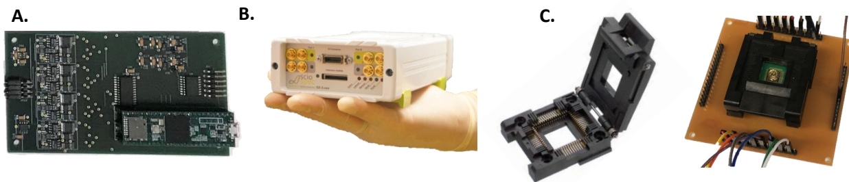
Figure 13: Measurement devices for electrical sensing, A. 4-Channel Portable Readout Module, B. Sciospec ISX-3 mini and C. Yamaichi IC-51 adapter.
